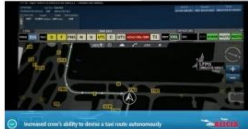
Airport Moving Map for the Cockpit
